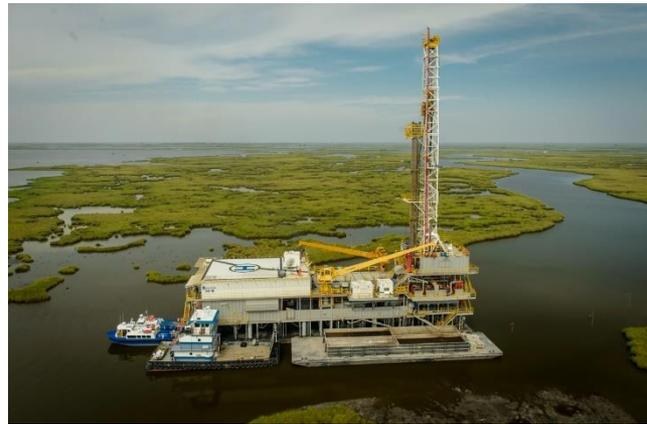
*Shallow-draft barge drilling rig*
