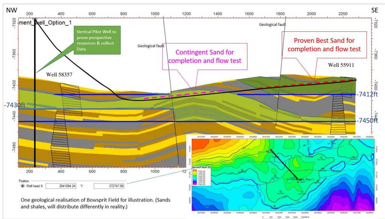
Figure 1 - Vertical Pilot hole and Horizontal Well Path
