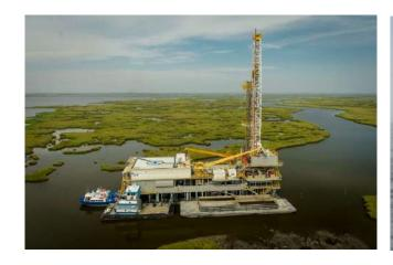
Shallow-draft barge drilling rig
