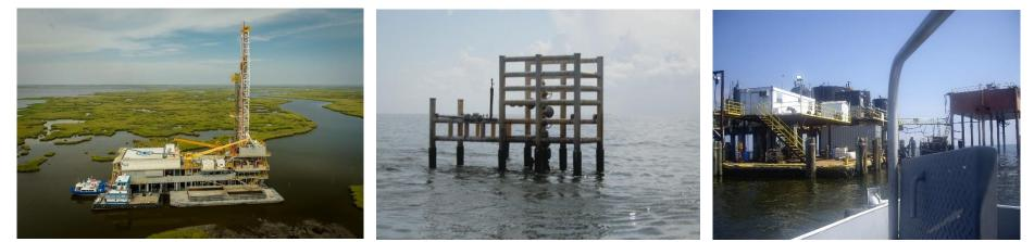
Shallow-draft barge drilling rig
