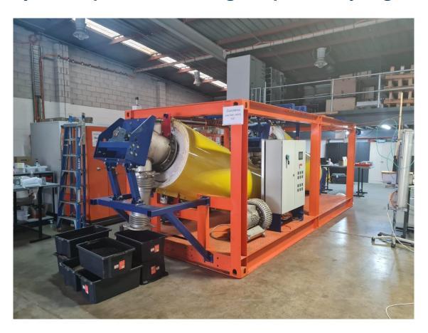
The modular Hydrogen units are scalable and can operate on multiple different feedstocks enabling them to be deployed over a range of different industries.
