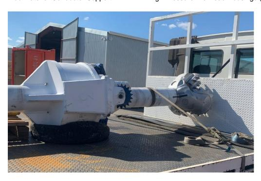
Hole Opener 26" Bit x 42" Hole Opener
