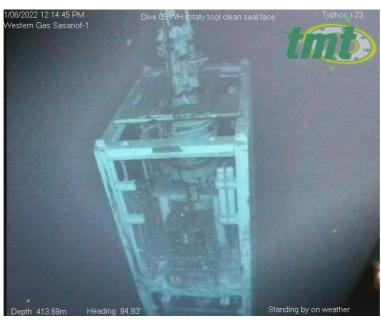
Blow out preventer being deployed towards the seabed.
